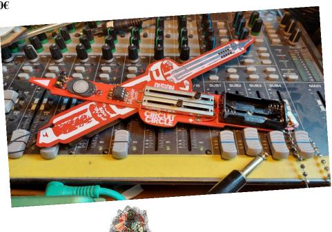
The "SUPALOOPA" is a standalone looping sounddevice based on the ISD 1820 board. With added pitch, in and output jack 6,3mm and an integrated speaker it is a fun device to bring some funky field recording sounds in your diy setup.
