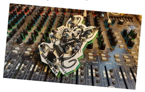
The "SillySolderIronSynth" ist he ultimate nerdy synth device. How cool ist that.. you can solder a solderiron...boom! It based on a attiny microcontroler and come along with nice and chaotic code with weird 8-bit noises, two sliders, a little speaker and 3.5mm jack out.
